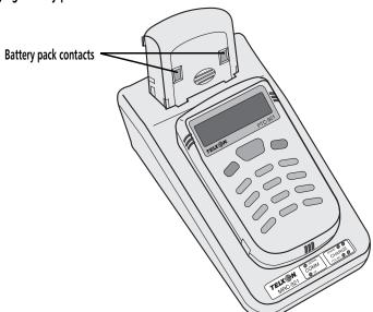
If the PTC bay is a trickle charger, its green LED will never light. The cradle does not indicate a full-charge state.
